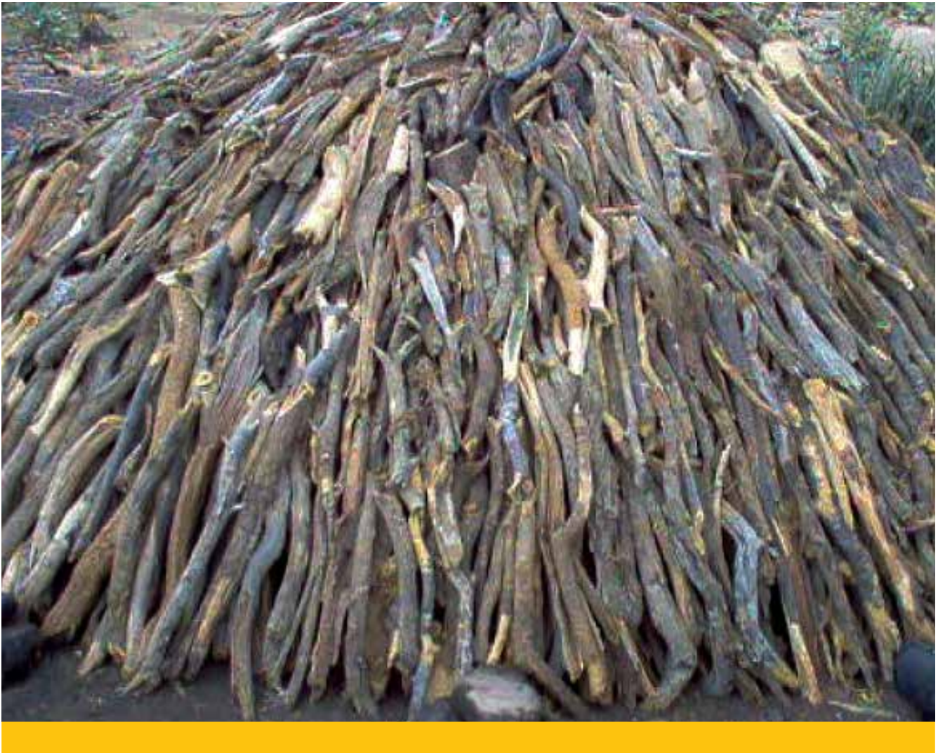
Circular kiln before being covered for artisanal charcoal production. Taken from Alzuru, A. I. (2005) Cited previously.
